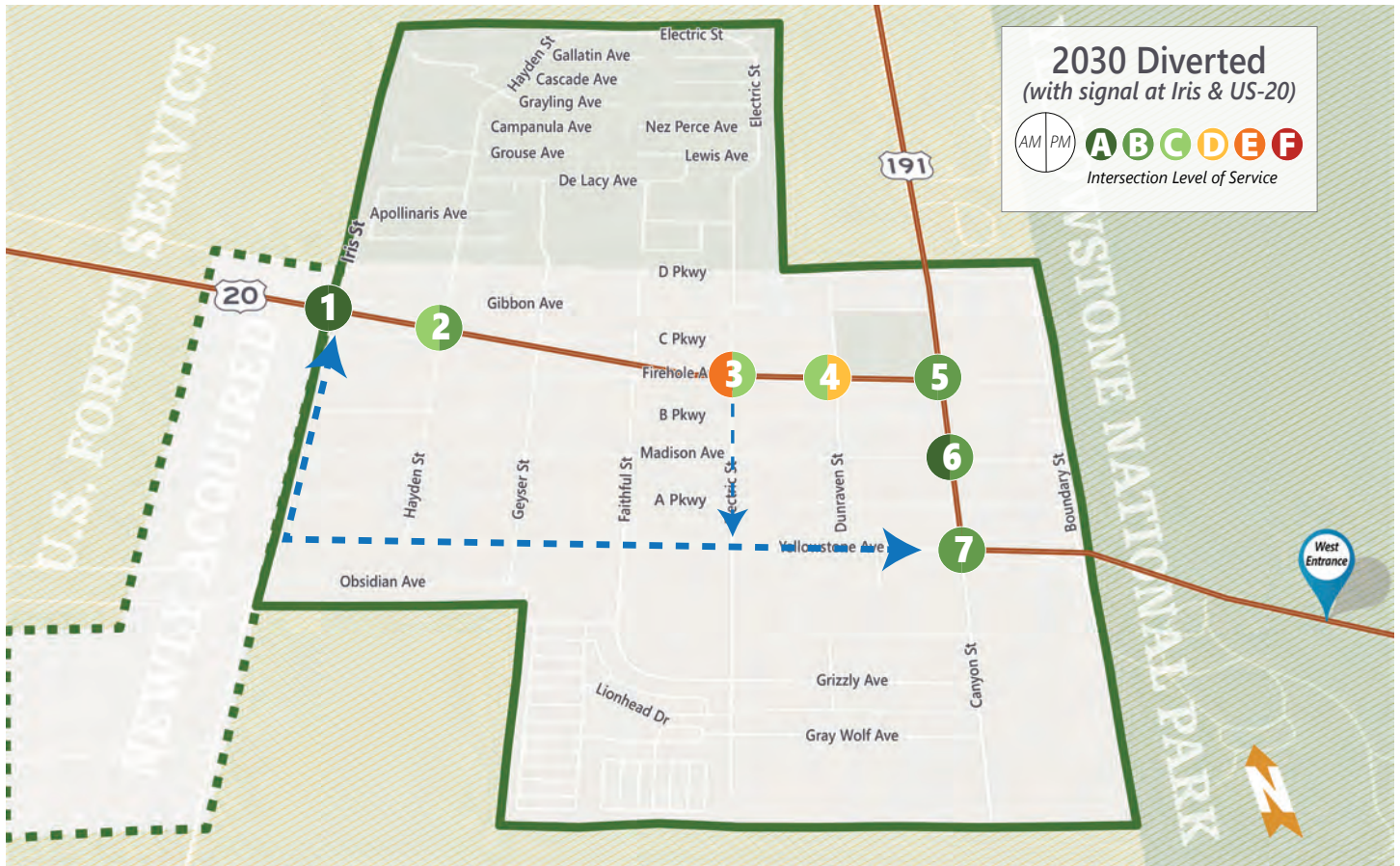
Figure 13: 2030 Diverted Roadway Alternative
