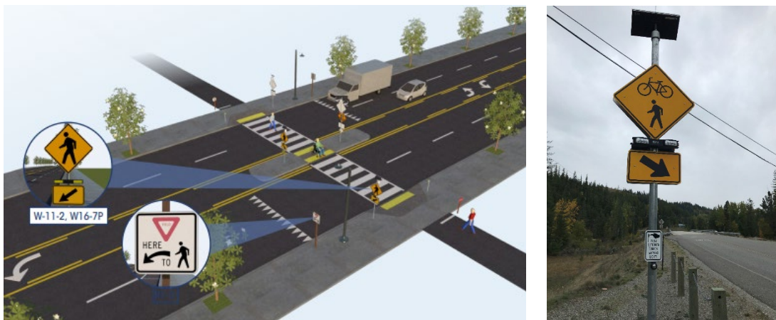
Figure 6. Example RRFB design for a four lane road and photo of an installed RRFB
